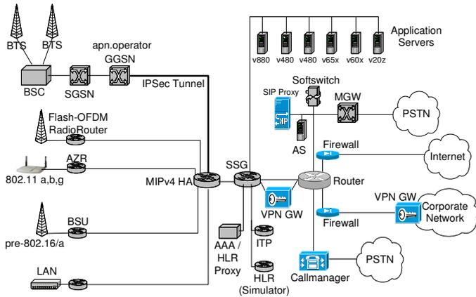
**Figure 2: overall testbed topology**
