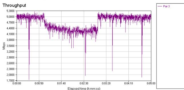
Figure 11: single-interval microwave interference on 802.11b
