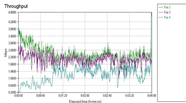
**Figure 8: throughput convergence in multi-user environments with BT**
