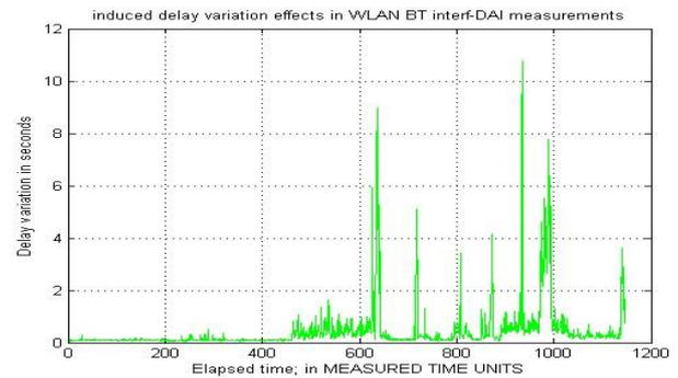
Figure 12: delay variations and increase due to BT interference
