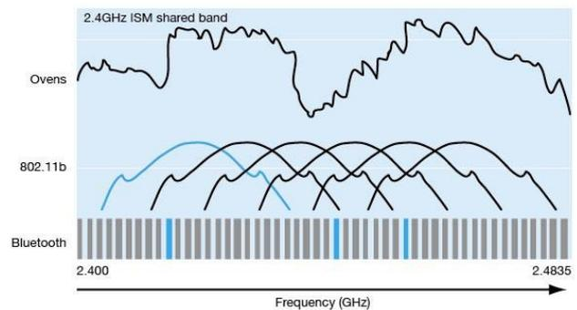
**Figure 4: ISM band with interfering technologies**
