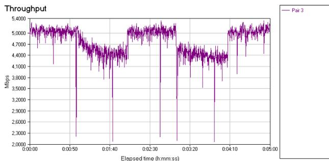
Figure 10: two-interval microwave interference on 802.11b
