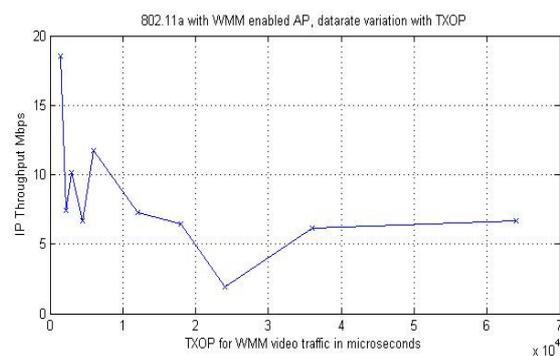
**Figure 7: 802.11a with WMM throughput change for fixed payload and increasing TXOP for video traffic**
