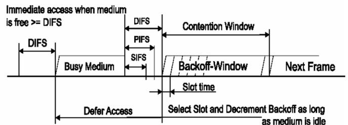
Figure 6: basic 802.11e mechanism
