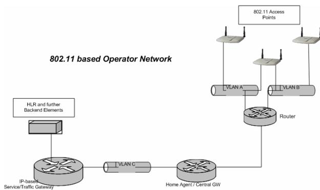
**Figure 3: topology of our WLAN-based network operator**
